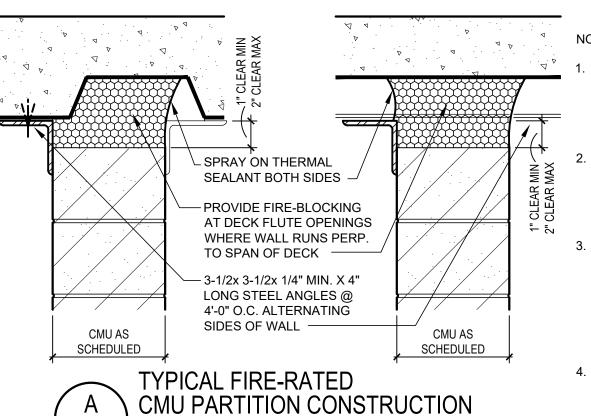
DECK FLUTE **OPENINGS WHERE** WALL RUNS PERP. TO SPAN OF DECK. 2. DO NOT ANCHOR VERTICAL STUDS TO TOP RUNNER. ALLOW FOR STRUCTURAL SLAB DEFLECTION.
