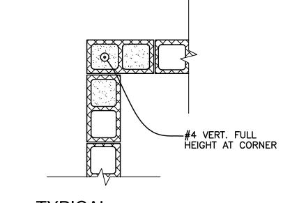
**TYPICAL** REINFORCING AT CORNERS SCALE : 3/4" = 1'-0"
