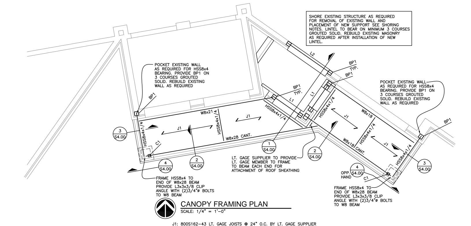
TYPICAL ROOF SHEATHING IS 5/8" PLYWOOD. PROVIDE ROOF CLIPS TYPICAL AT PANEL EDGES BETWEEN TRUSSES. STAGGER PLYWOOD JOINTS BETWEEN ROWS OF SHEATHING (OFFSET 4'-0" EACH ROW) ATTACH TO LT. GAGE TRUSSES WITH #10 TEK SCREWS 6" O.C. AT EDGES AND 12" O.C. IN THE FIELD
