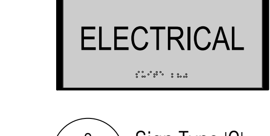
3 Sign Type 'C' N.T.S. NOTES: 1. SEE SIGN TYPE 'A' FOR TYPICAL NOTES & DIMENSIONS 2. PROVIDE (2) SIGNS MOUNTED TO SOLID WALLS 3. LOCATE IN FIELD PER ARCHITECT 4. LOCATE PER MOUNTING DETAIL 1
