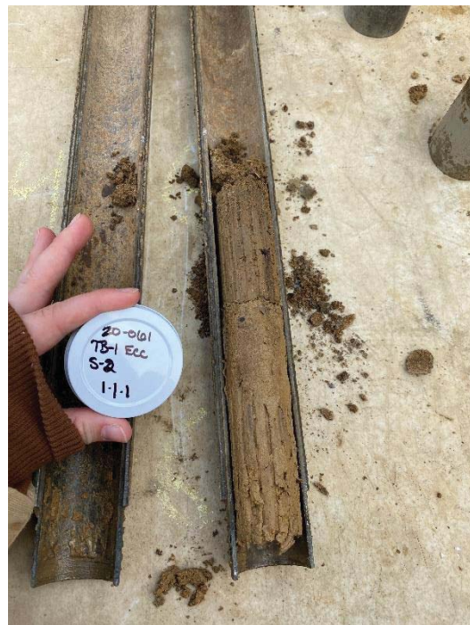
Figure 5 – TB-1 Sloan, Sample S-2 (5ft) – Very Loose Clayey Sand
