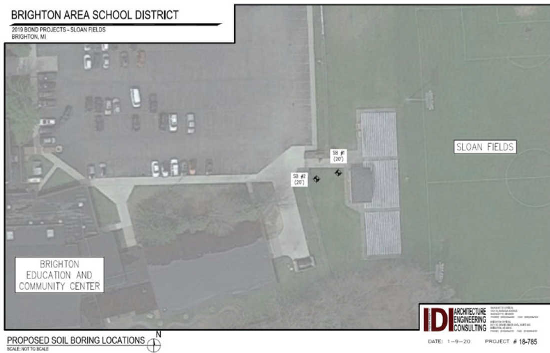
Figure 1 - IDI provided soil boring location plan
