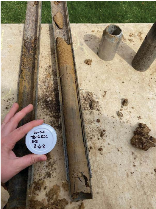
Figure 4 – TB-2 Sloan, Sample S-5 (15ft) – Very Stiff Silty Clay
