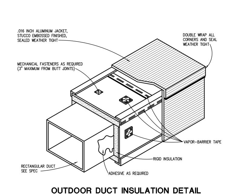
OUTDOOR DUCT INSULATION DETAIL
