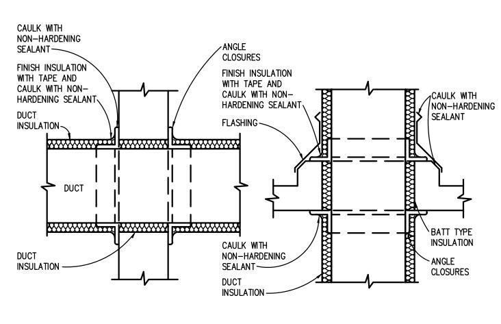
VERTICAL OR HORIZONTAL (NON FIRE RATED ASSEMBLY) DUCT PENETRATION DETAIL
