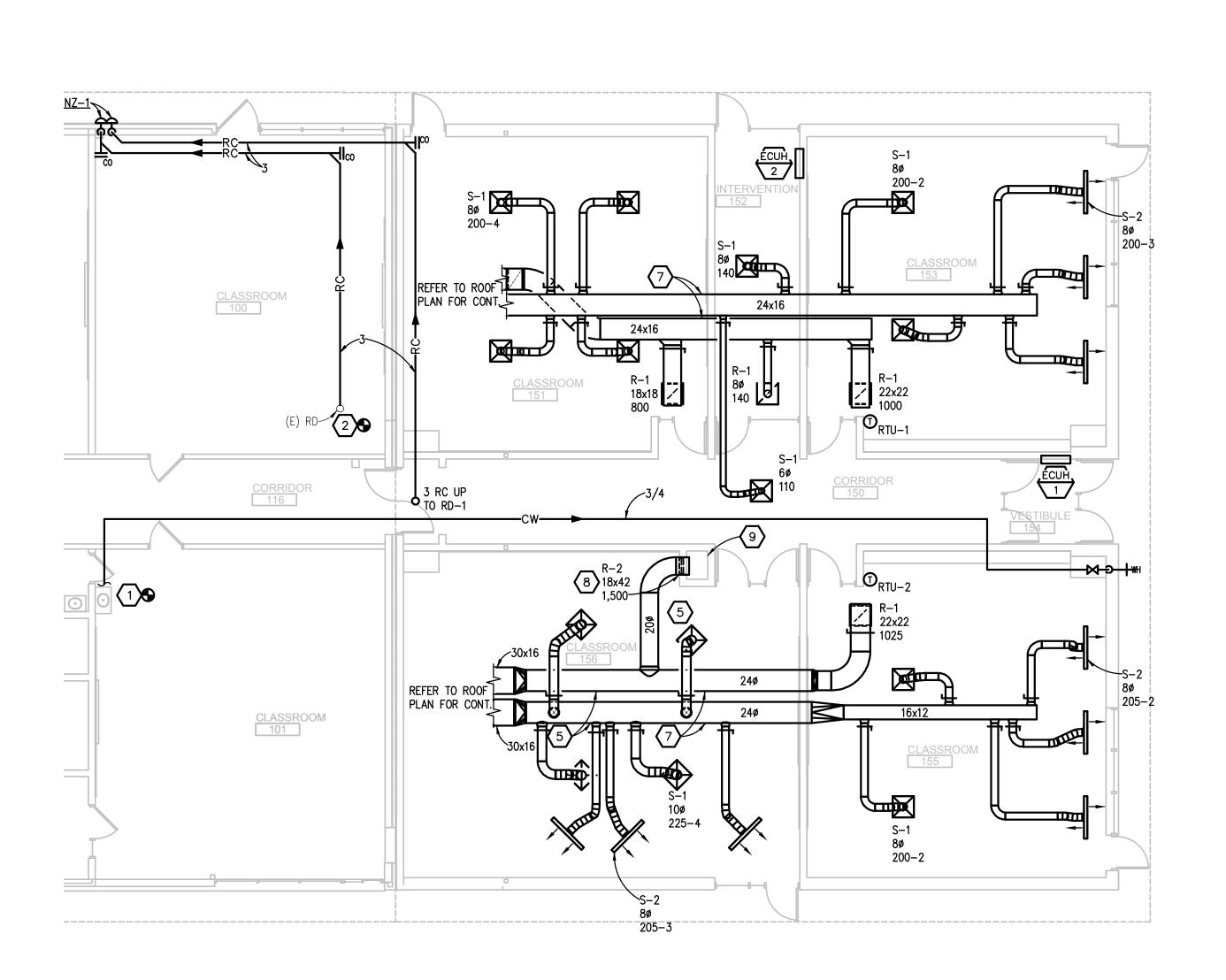
PARTIAL FIRST FLOOR MECHANICAL NEW WORK PLAN SCALE: 1/8" - 1' - 0"
