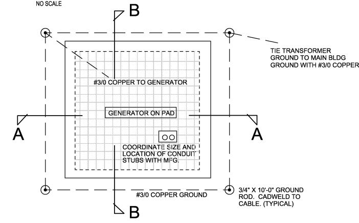
CONCRETE PAD TO BE 4,000PSI CONCRETE 8" THICK. SIZE TO BE 12" LARGER THAN GENERATOR IN ALL DIMENSIONS. PROVIDE #4 REBAR ON 12" CENTERS IN BOTH DIRECTIONS. PAD TO BE 2" ABOVE GRADE WITH 1" X 1" X 45 DEGREE CHAMFER ON TOP EDGE ALL THE WAY AROUND. SET ON A MINIMUM OF 12" DEPTH OF CLEAN COMPACTED SAND.
