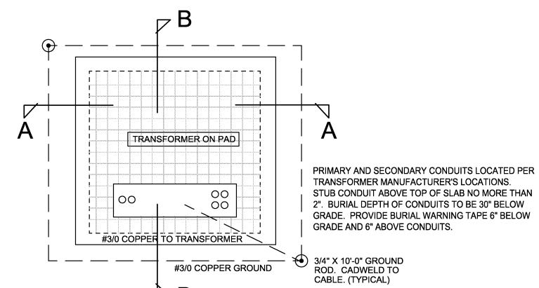
CONCRETE PAD TO BE 4,000PSI CONCRETE 8" THICK SIZE TO BE 6" LARGER THAN TRANSFORMER IN ALL DIMENSIONS. PROVIDE #3 REBAR ON 12" CENTERS IN BOTH DIRECTIONS. PAD TO BE 2" ABOVE GRADE WITH 1" X 1" X 45 DEGREE CHAMFER ON TOP EDGE ALL THE WAY AROUND. SET ON A MINIMUM OF 12" DEPTH OF CLEAN COMPACTED SAND.
