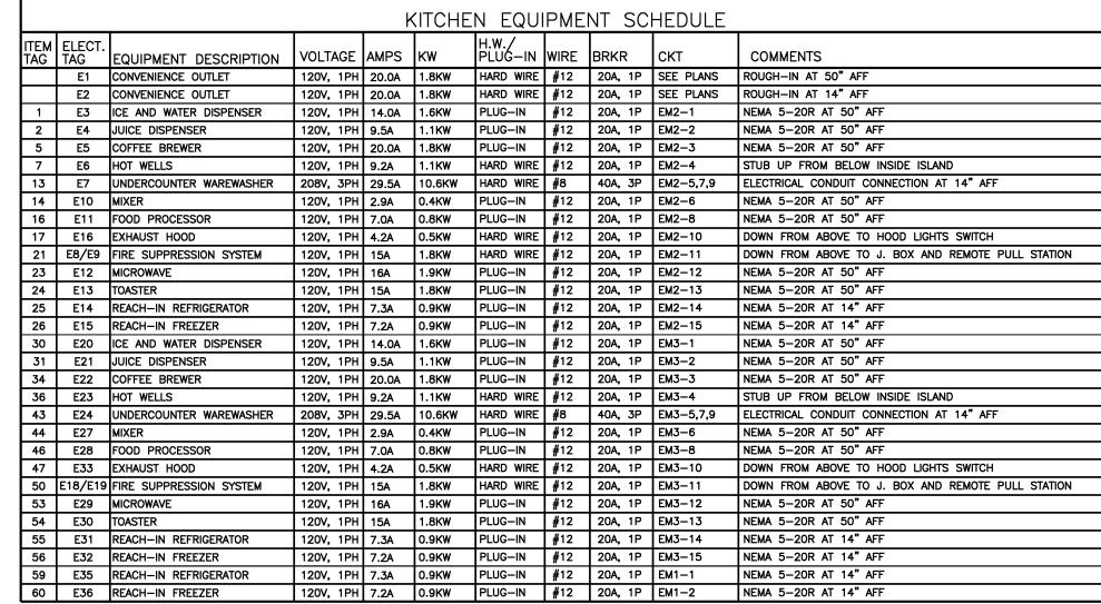
REFERENCE KITCHEN CONSULTANT'S DRAWINGS FSE-3 AND PRODUCT CUT-SHEETS OF ABOVE EQUIPMENT FOR ALL INSTALLATION REQUIREMENTS ROUGH-IN HEIGHTS AND ANCILLARY WIRING REQUIREMENTS. E.C. TO INSTALL AND PROVIDE WIRING OF CONTROL PANELS, HOODS, FIRE SUPRESSION, CONTROL VALVES, ETC. AS REQUIRED FOR A COMPLETE AND OPERATIONAL SYSTEM. COORDINATE WITH FSES DRAWINGS.
